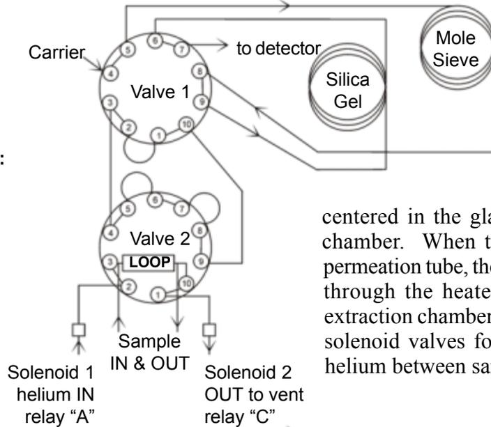
centered in the glass tube which functions as the extraction chamber. When the transformer oil is pumped through the permeation tube, the dissolved gases therein selectively permeate through the heated (70°C) membrane into the surrounding extraction chamber. Plumbed to the dual 10-port valves are two solenoid valves for purging the gas extraction chamber with helium between sample injections, to prevent carryover.
