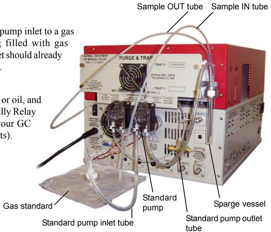
4. To sample the standard you've created with the tedlar bag and liquid-filled sparge tube: attach the SAMPLE IN and OUT tubes to the STANDARD IN and OUT tubes on the top of the sparge vessel.
