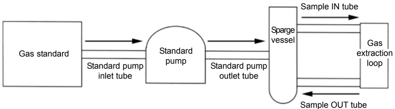
5. The extracted standard will return to the sparge tube to be regenerated for subsequent analysis.
