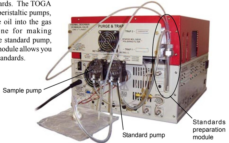
The gas extraction loop uses dual 10-port gas sampling valves with solenoids for helium purge/flush. The TOGA GC may be equipped with a TCD detector, an HID detector, or both.
