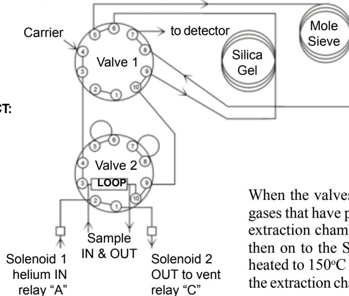
Valve 1 is plumbed to the Molecular Sieve 13X column, then to the Silica Gel column. Valve 2 is plumbed to the gas extraction loop. While the transformer oil is being pumped through the gas extraction loop, both valves are in the LOAD position. During this time, the gases dissolved in the transformer oil are extracted by selective permeation through the membrane.
