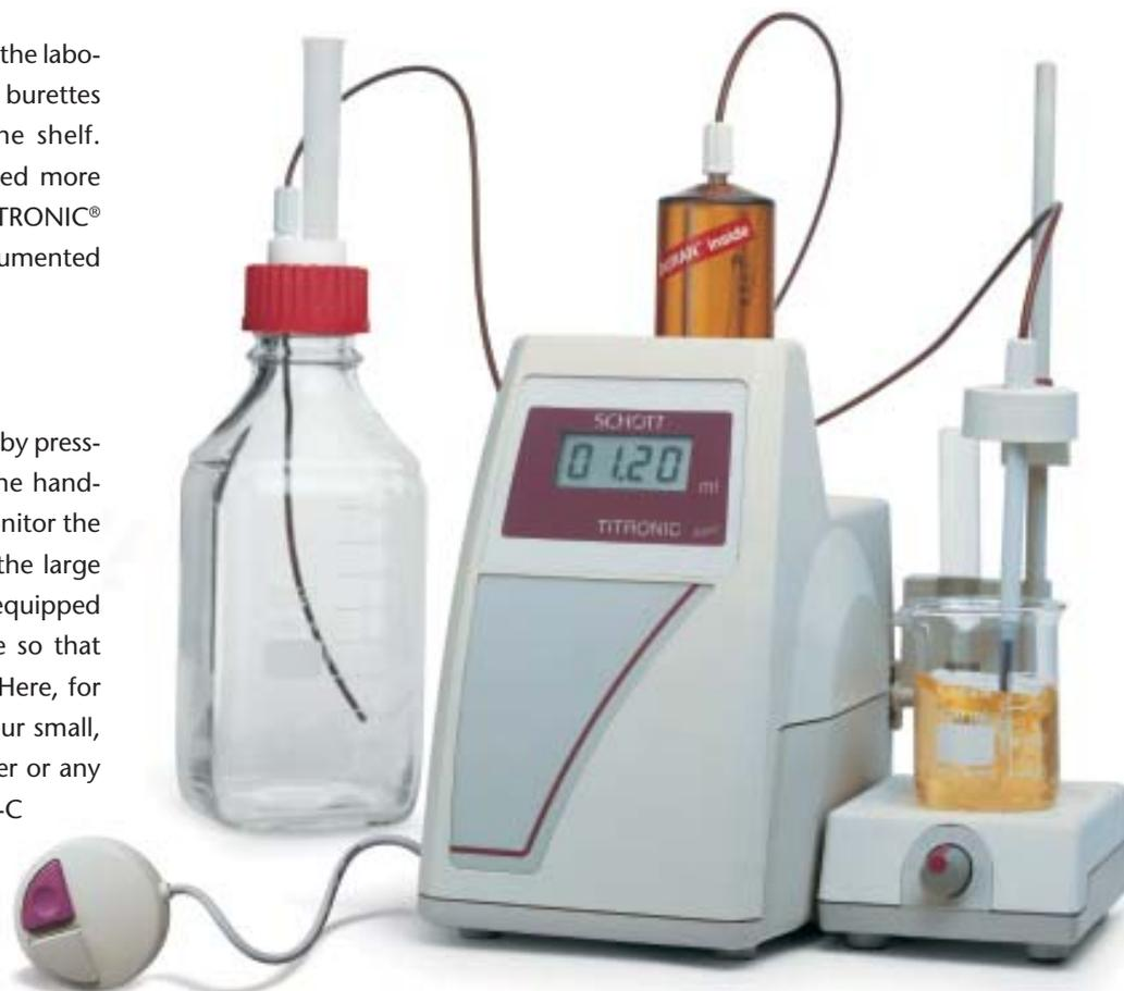
The complete workplace: precision analysis with no shaky compromises. With 8000-step resolution, precision glass cylinder with UV-protection, motor-controlled 3/2-way valve of extremely resistant PTFE/ETFE and an interface for documentation of the results. It's better to be on the safe side! (The bottle set must be ordered separately as an accessory.)
