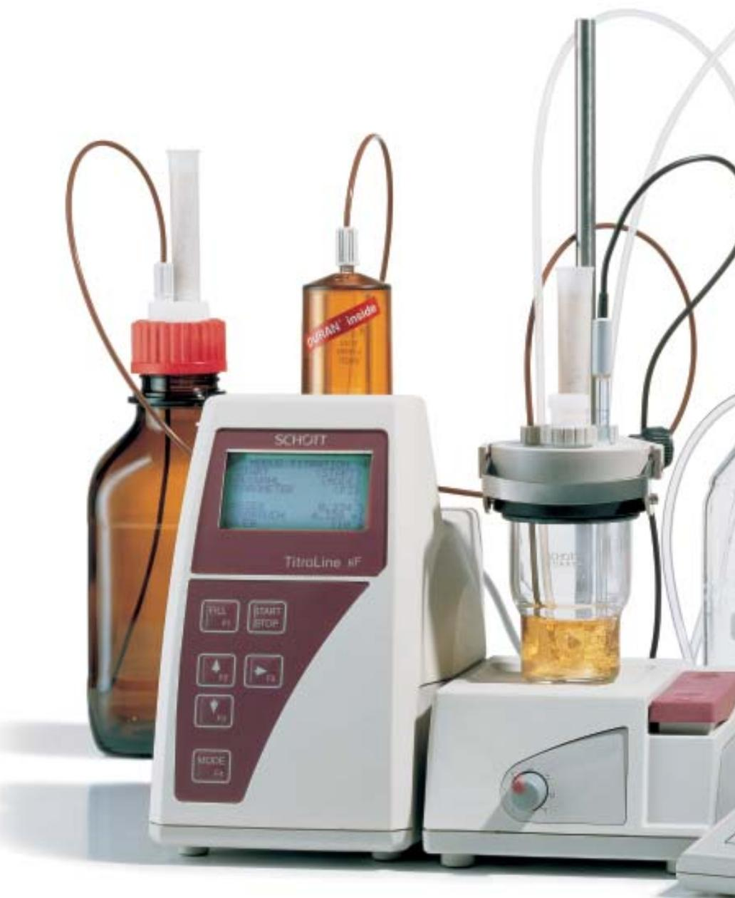
The TitroLine KF includes everything you need for water analysis according to Karl Fischer. The scope of supply includes the titrator, reagent bottle, titration stand TM KF, titration vessel, electrode and a starter kit (6 syringes with tubular needles, molecular sieve and three ampoules with a water standard specification). The waterproof mini keyboard TZ 2825 is available as an optional extra.
